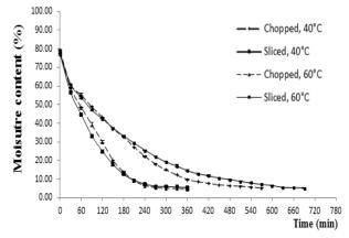
Figure 1. The drying curves of chopped and sliced garlic using hot air oven at 40°C and 60°C
