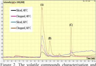
Figure 2. The volatile compounds characterisation and intensity of dried garlic powder using GC-FID; (A) allyl methyl sulfide, (B) diallyl disulfide, and (C) diallyl trisulfide
